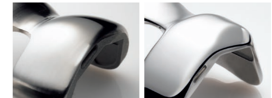
Example: highly polished surface, Ra 0.01 \mu m
