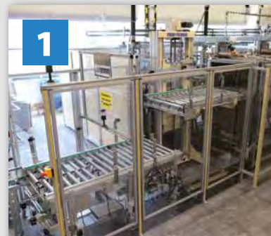
Detail lifting/lowering station
